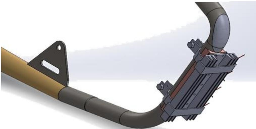
Thermoelectric Generator on Bike Exhaust Manifold
